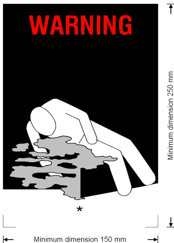
Asphyxiation warning mark for wagons and containers
